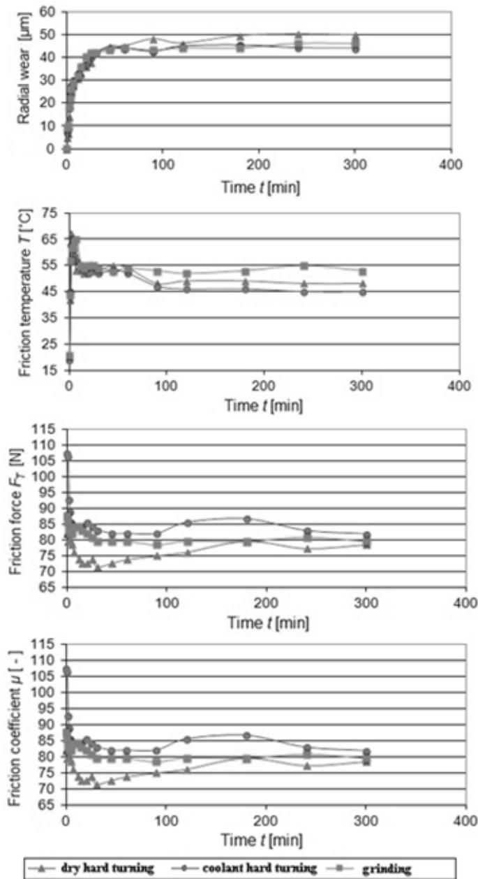
Fig. 4. graphical dependences of complex tribological characteristics when hard turning and grinding of tool hardened steel CT120.
