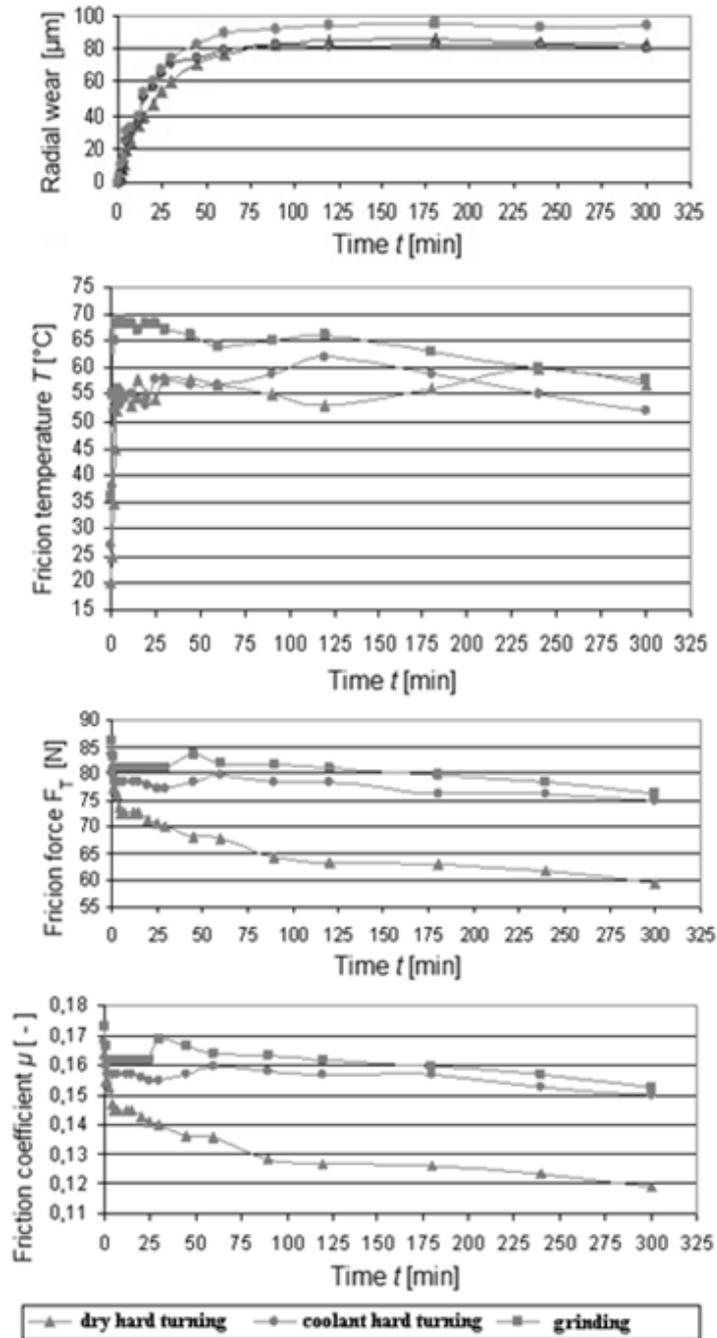
Fig. 3. graphical dependences of complex tribological characteristics when hard turning and grinding of bearing hardened steel 102Cr6.
