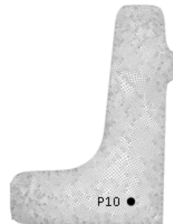
Fig. 2. Model of real forging created using FEM simulation- cross section with reference point for material-technological mode.
