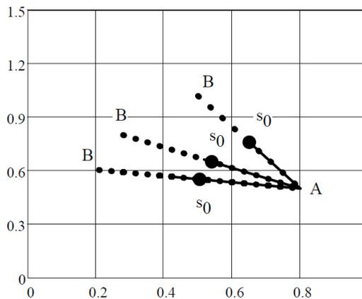
Fig. 7. The berry (continuous line) and the belt (dotted line) trajectories,  $s_0$  location (large dot): 1)  $\beta = 10^\circ$ , 2)  $\beta = 30^\circ$ , 3)  $\beta = 60^\circ$ ;  $f = 0.01$ ,  $v_k = 1m/s$ ,  $s_0 = 0.3m$ ,  $s'_0 = 0.5m/s$ .
