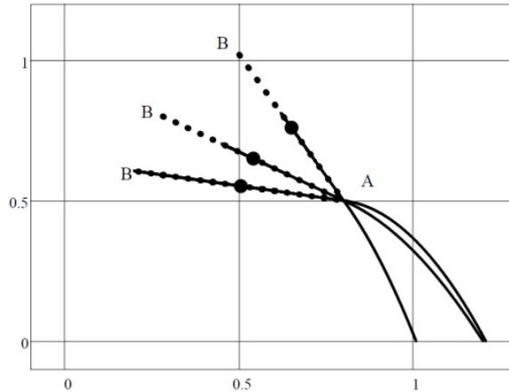
Fig. 8. Berry’s entire trajectory on the belt and through the air, when 1)  $\beta = 10^\circ$ , 2)  $\beta = 30^\circ$ , 3)  $\beta = 60^\circ$ ;  $v_k = 1m/s$ ,  $f = 0.01$ ,  $s_0 = 0.3m$ ,  $s'_0 = 0$ .
