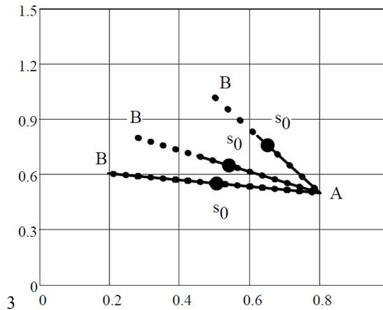
Fig. 6. The berry (continuous line) and the belt (dotted line) trajectories,  $s_0$  location (large dot): 1)  $\beta = 10^\circ$ , 2)  $\beta = 30^\circ$ , 3)  $\beta = 60^\circ$ ;  $f = 0.01$ ,  $v_k = 1m/s$ ,  $s_0 = 0.3m$ ,  $s'_0 = 0$ .
