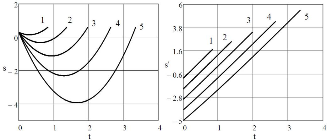
Fig. 4. Left: berry displacement along conveyor belt. Right: berry velocity along conveyor belt. Corresponding different velocities of the conveyor belt: 1)  $v_k = 1\text{m/s}$ , 2)  $v_k = 2\text{m/s}$ , 3)  $v_k = 3\text{m/s}$ , 4)  $v_k = 4\text{m/s}$ , 5)  $v_k = 5\text{m/s}$ ;  $\beta = 20^\circ$  and  $f = 0.01$ .
