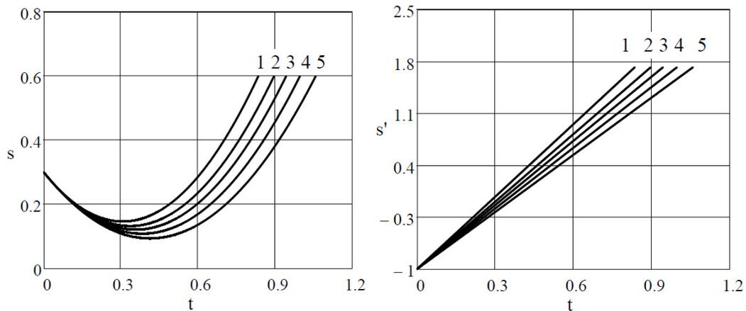
Fig. 5. Left: berry displacement along conveyor belt. Right: berry velocity along conveyor belt. Corresponding different friction coefficient between berry particle and conveyor belt: 1)  $f = 0.01$ , 2)  $f = 0.05$ , 3)  $f = 0.1$ , 4)  $f = 0.15$ , 5)  $f = 0.2$ ;  $v_k = 5\text{m/s}$  and  $\beta = 20^\circ$ .
