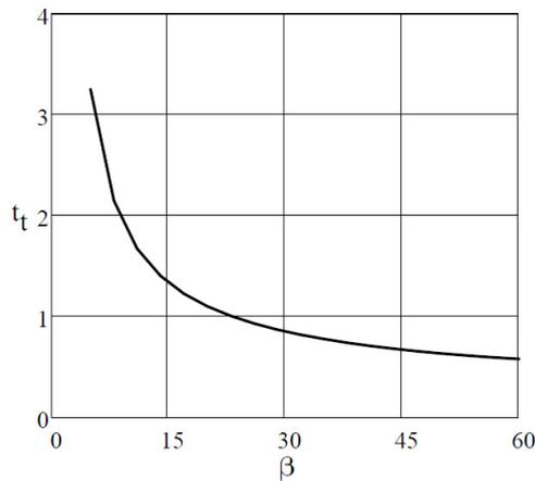
Fig. 9. Total time of berry motion depending on inclination angle  $\beta$  of conveyor belt if  $v_k = 1m/s$ ,  $f = 0.01$ ,  $s_0 = 0.3m$ ,  $s'_0 = 0$ .
