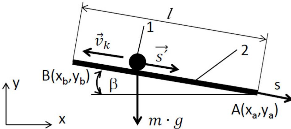
Fig. 2. The computational scheme of belt conveyor: 1 – berry particle, 2 – conveyor belt between points AB, l – width of the belt (distance between points AB),  $v_k$  – velocity of the conveyor belt,  $s$  – axis, with origin at the point B along the conveyor belt,  $s'$  – berry’s velocity,  $\beta$  – inclination angle of the conveyor belt,  $m$  – berry particle mass,  $g$  – acceleration of gravity.
