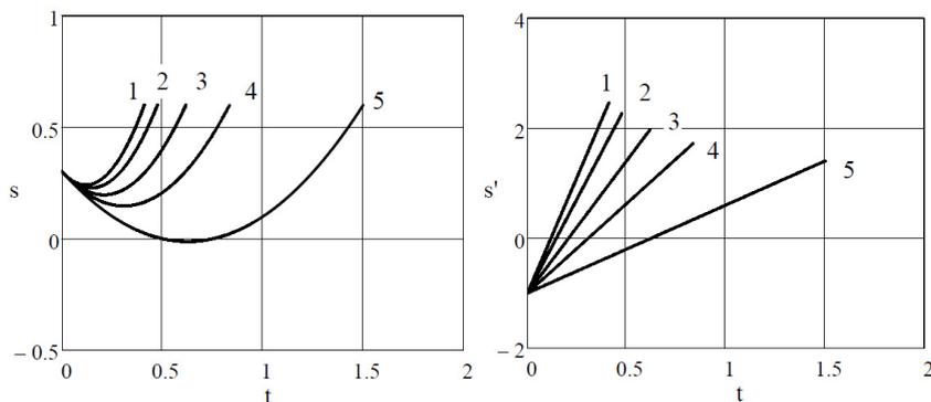
Fig. 3. Left: berry displacement along conveyor belt. Right: berry velocity along conveyor belt. Corresponding different inclination angles of the conveyor belt: 1)  $\beta = 60^\circ$ , 2)  $\beta = 45^\circ$ , 3)  $\beta = 30^\circ$ , 4)  $\beta = 20^\circ$ , 5)  $\beta = 10^\circ$ ;  $v_k = 5 \text{ m/s}$  and  $f = 0.01$ .
