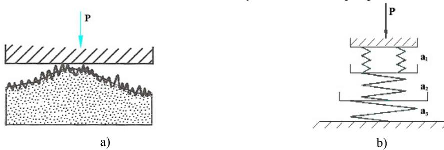
Fig.1. Scheme of contact: a) whole scheme; b) scheme of spring principal.
