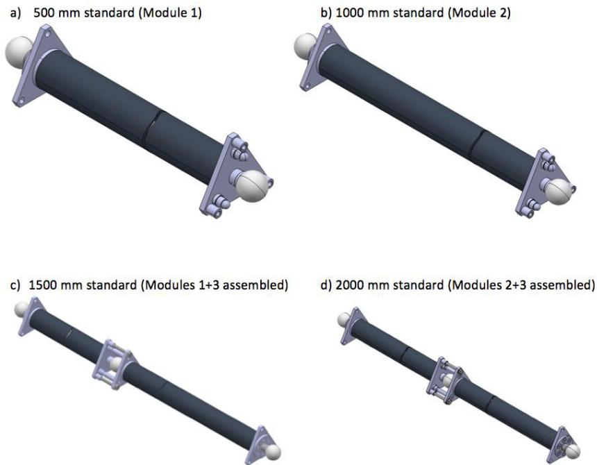
Fig. 1. Conceptual design of the standard.
