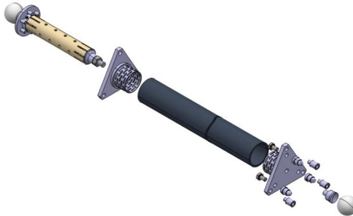
Fig. 2. Design of modules 1 and 2.
