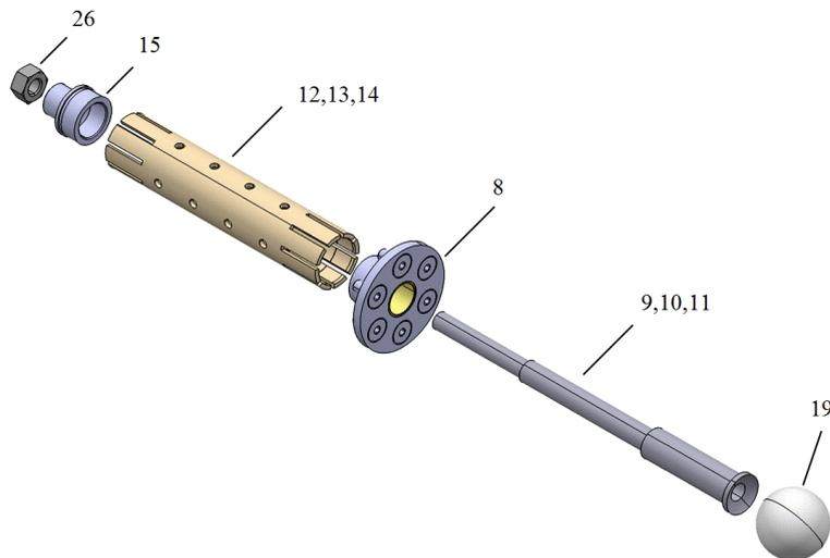
Fig. 3. Thermal expansion compensator.
