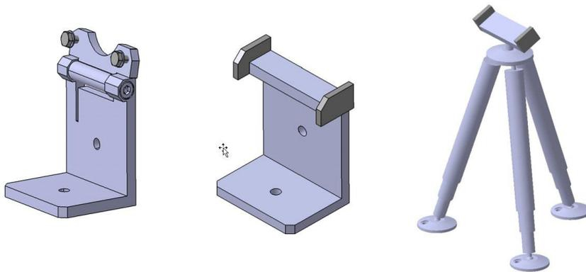
Fig. 5. Supporting and fixing elements for positioning the standard within machine-tool volume.
