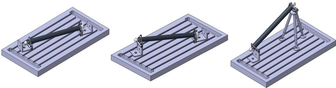
Fig. 6. Examples of positioning the standard within machine-tool volume.
