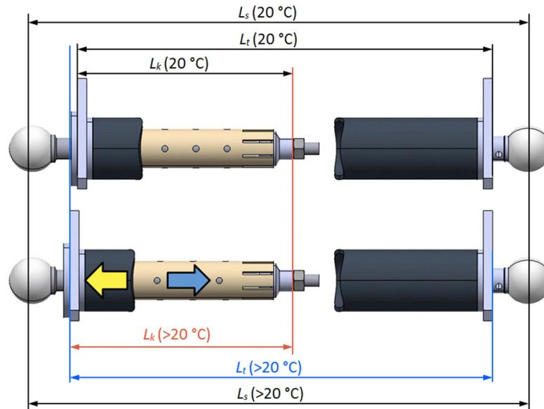
Fig. 4. Thermal expansion compensator – principle of operation.
