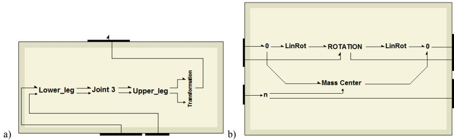
Fig. 4. Bond graph component of legs **Leg i** ( $i=1,2,..6$ ): (a) the first level of decomposition; (b) structure of **Lower\_leg** or **Upper\_leg**.
