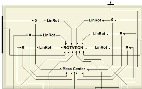
Fig. 5. Bond graph component of moving platform.
