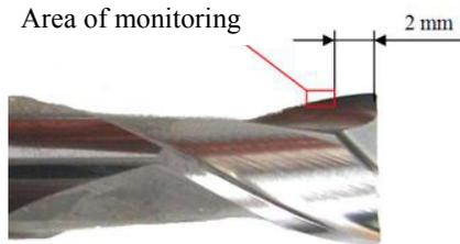
Fig. 1. Area of monitoring on the cutting edge.
