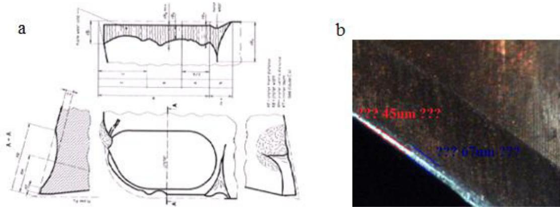
Fig. 12. (a) Evaluation of the tool wear according to the standard; (b) Conventional method of measuring tool wear [7].
