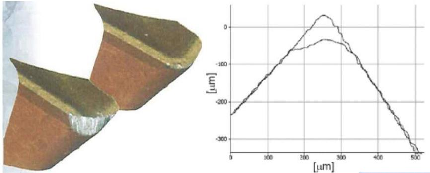
Fig. 15. Evaluation of tool wear through contours of the new and worn tools [3].
