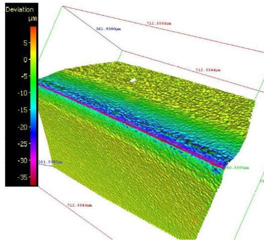
Fig. 14. Evaluation of tool wear though difference analysis.
