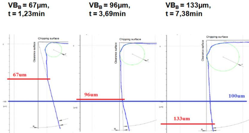
Fig. 13. Measuring tool wear on IFM G4.
