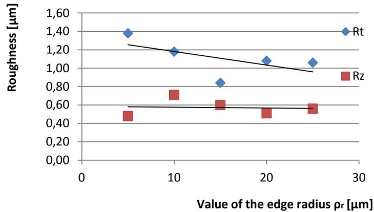
Fig. 10. Roughness in relation to radius of the cutting edge.
