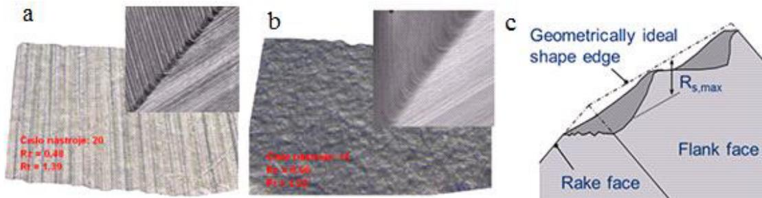
Fig. 11. (a) Surface after grinding (on the left) (b) after drag finishing (in the middle); (c) Chipping – roughness of the cutting edge.
