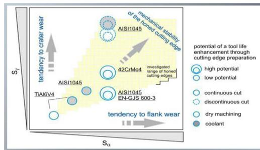
Fig. 8. Influence of the size  $S_\gamma$  and  $S_\alpha$  on tool wear [2].
