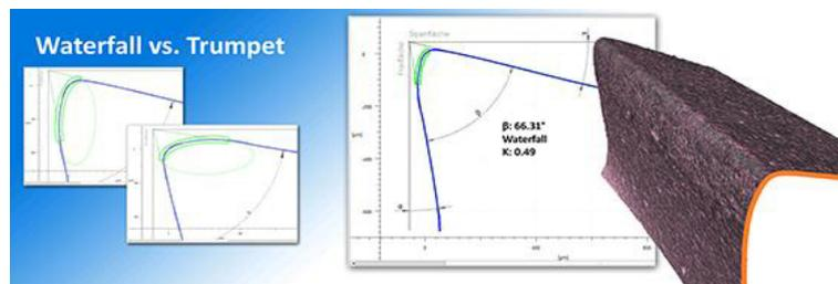
Fig. 3. Elliptical shapes of the cutting edge.
