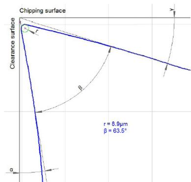
Fig. 9. Incorrect interleaving of tangents to the measured radius.
