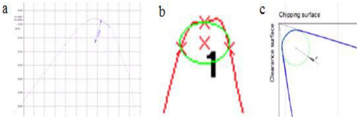
Fig. 2. Results of cutting edge radius from tactile device, confocal microscope, and IFM G4.
