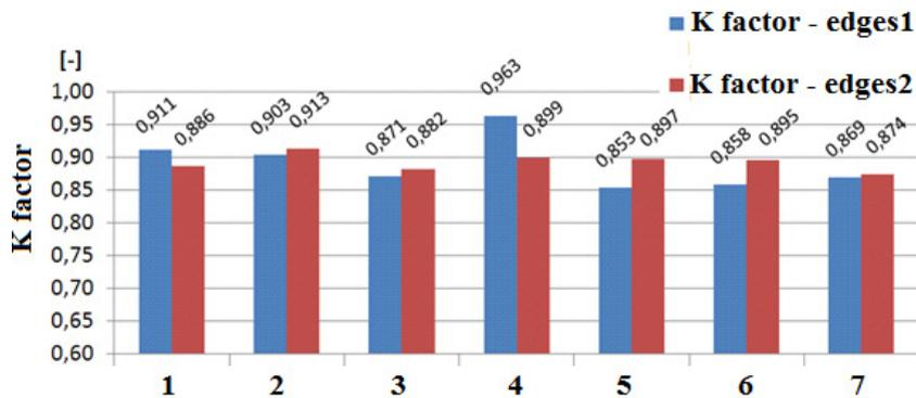
Fig. 6. Values of K factor for different modified tools.
