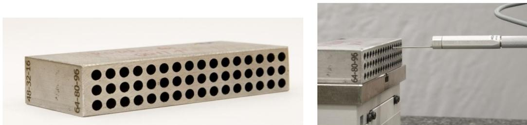
Fig. 5. (a) Measured piece with 96 holes (b) Roughness sensor approaching the hole for measurement.
