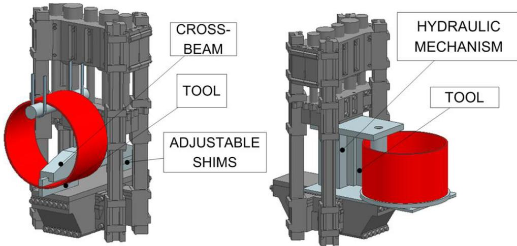
Fig. 2. Device for forging rings (left-variant 1, right-variant 2)
