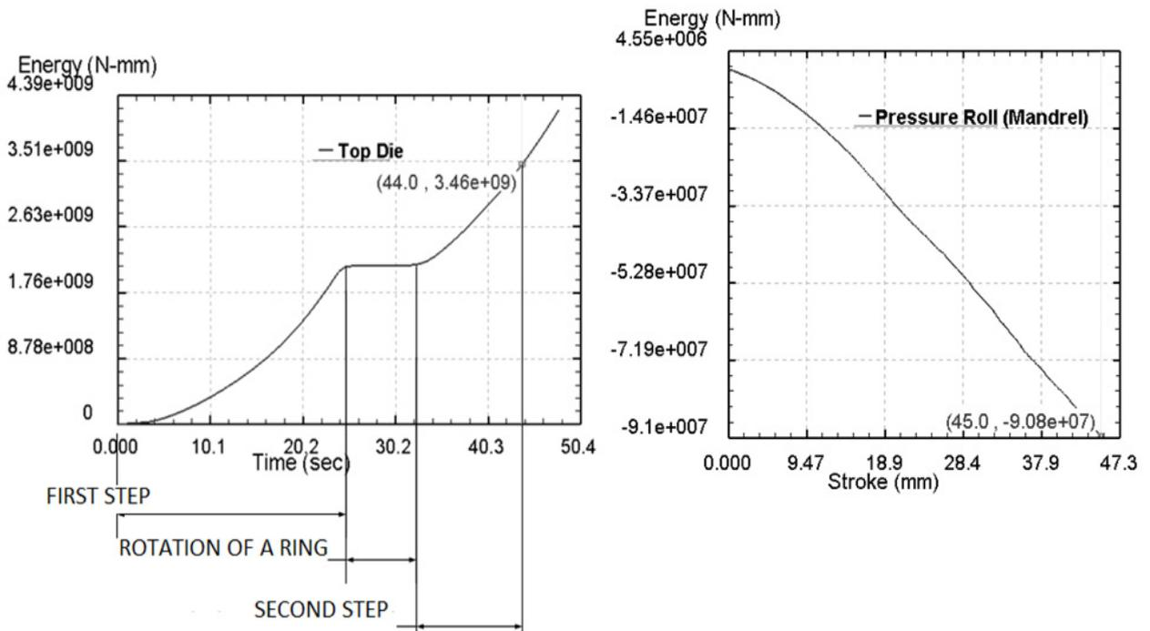
Fig. 4. Energy consumption during production (left-forging, right-rolling)
