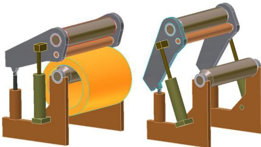
Fig. 3. Device for rolling rings.
