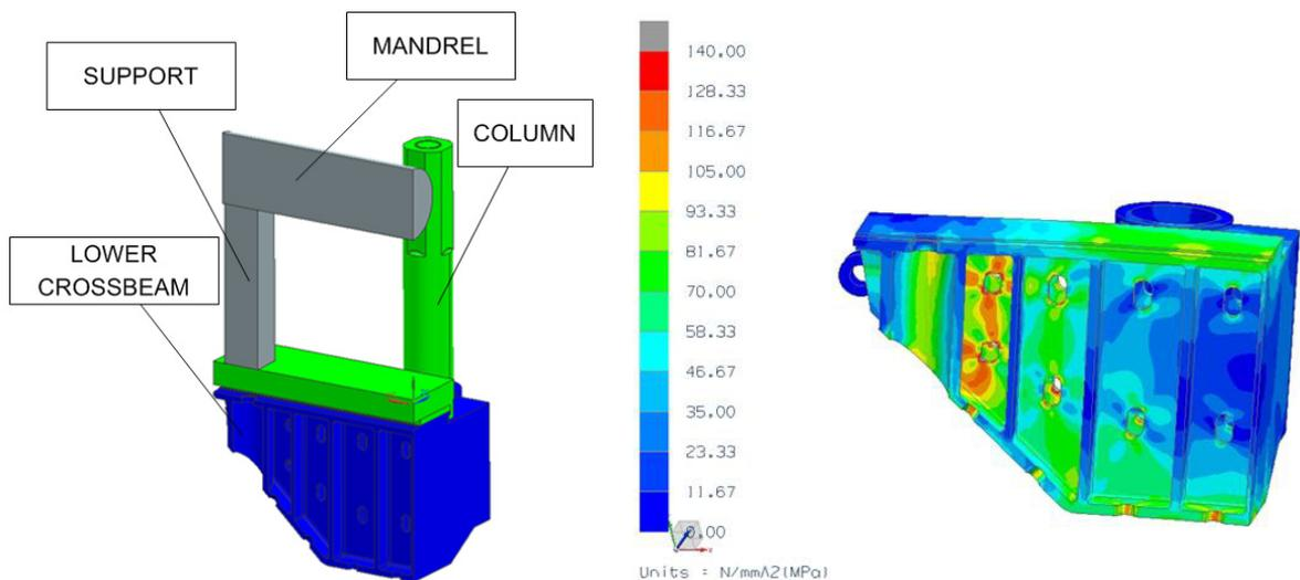
Fig. 5. Computational model and stress distribution in quarter model of lower crossbeam.
