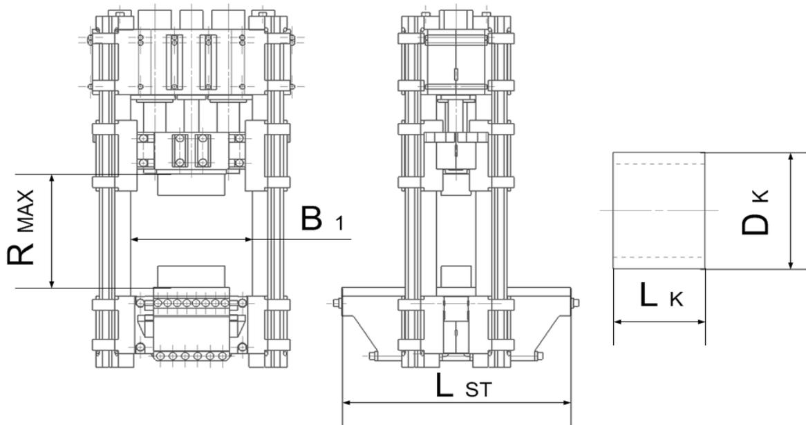
Fig. 1. Dimensions of hydraulic press and forged ring.
