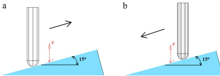
Fig. 3. (a) upward ramping; (b) downward ramping.
