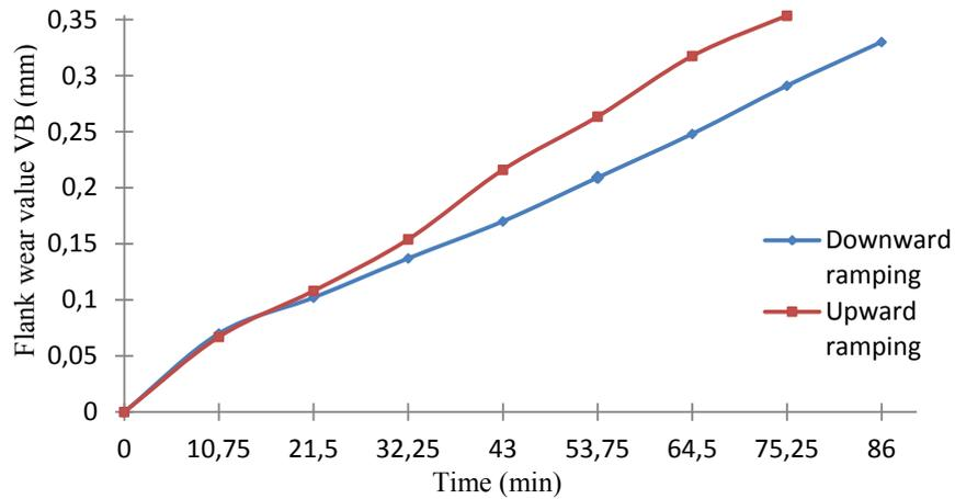
Fig. 6. the time dependence of flank wear.
