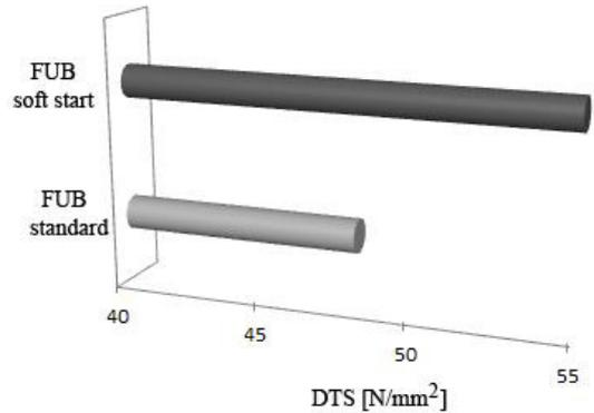
Fig. 19. Diametral tensile strength for FUB.
