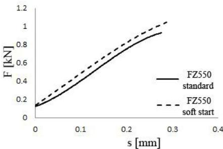
Fig. 14. F-s diagram in diametral tensile test for FZ550.
