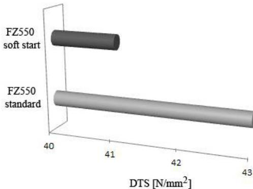
Fig. 20. Diametral tensile strength for FZ550.
