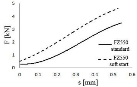
Fig. 11. F-s diagram in compressive test for FZ550.
