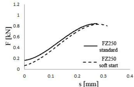
Fig. 15. F-s diagram in diametral tensile test for FZ250.
