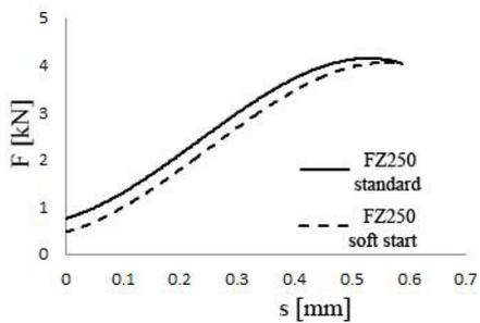
Fig. 12. F-s diagram in compressive test for FZ250.
