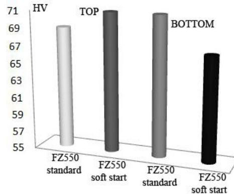
Fig. 23. Hardness test values for FZ550.
