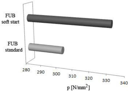
Fig. 16. Compressive strength for FUB.
