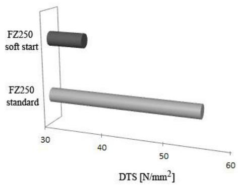
Fig. 21. Diametral tensile strength for FZ250.
