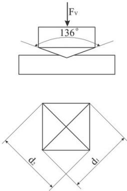
Fig. 8. Hardness test procedure.
