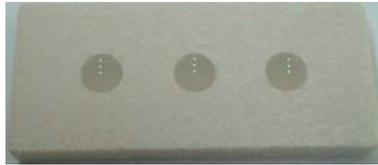
Fig. 7. Vickers hardness test specimens.
