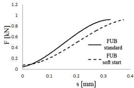
Fig. 13. F-s diagram in diametral tensile test for FUB.
