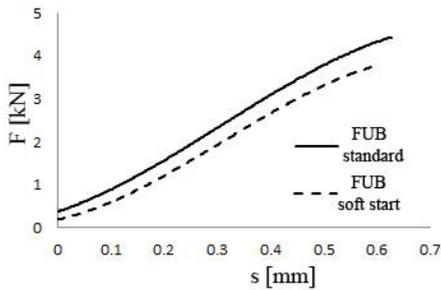
Fig. 10. F-s diagram in compressive test for FUB.
