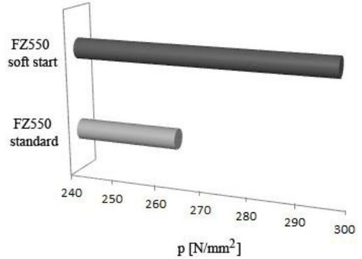
Fig. 17. Compressive strength for FZ550.
