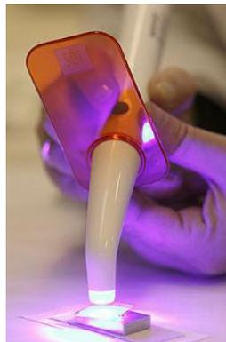
Fig. 2. Polymerization of the specimens by exposing to light of dental light-energy source [18].
