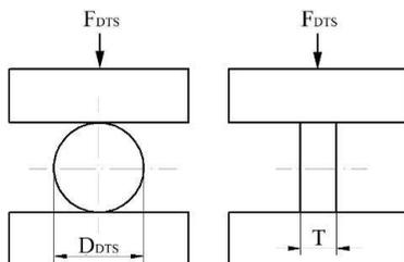
Fig. 5. Diametral tensile test procedure.
