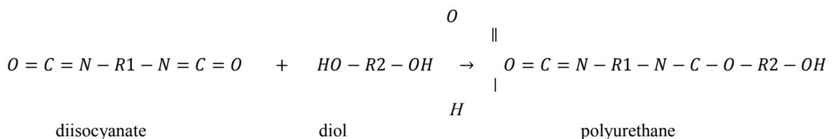
Fig. 1. Polyurethane synthesis [2].
