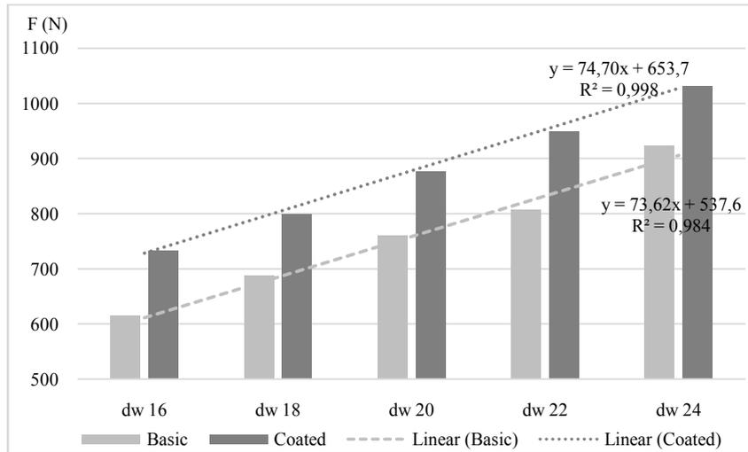
Fig.2. Breaking force (F (N)) of tested fabrics – basic and coated fabrics, where: dw – warp density (threads/cm).
