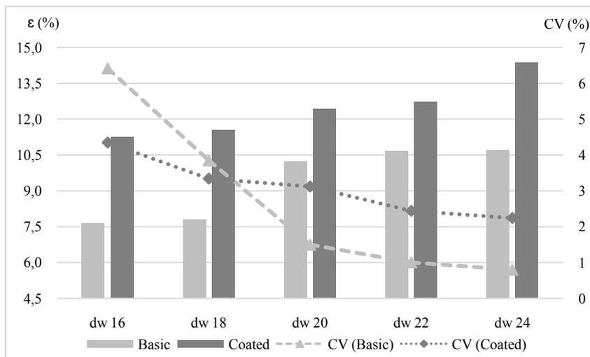
Fig.5. Elongation at break (ε (%)) during the ball bursting test of fabrics - basic and coated fabrics, where: dw – warp density (threads/cm).
