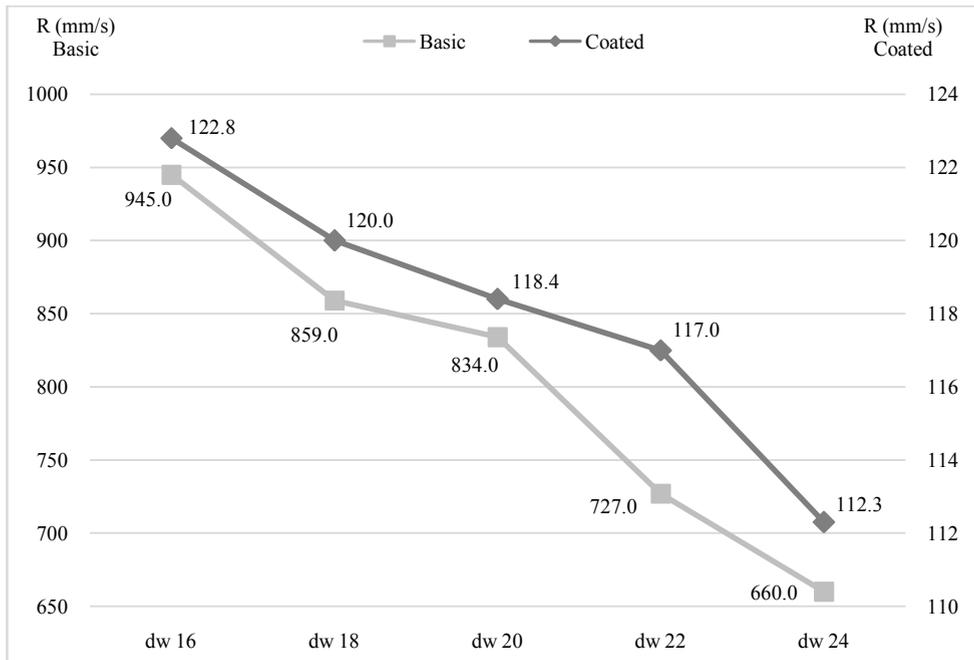
Fig.6. Fabric air permeability (R (mm/s)) - basic and coated fabrics, where: dw – warp density (threads/cm).
