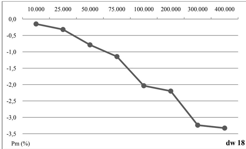
Fig.9. Abrasion resistance of coated fabric with warp density 18 threads/cm.
