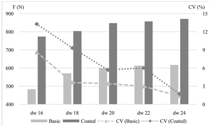
Fig.4. Bursting strength (F (N)) of tested fabrics - basic and coated fabrics, where: dw – warp density (threads/cm).
