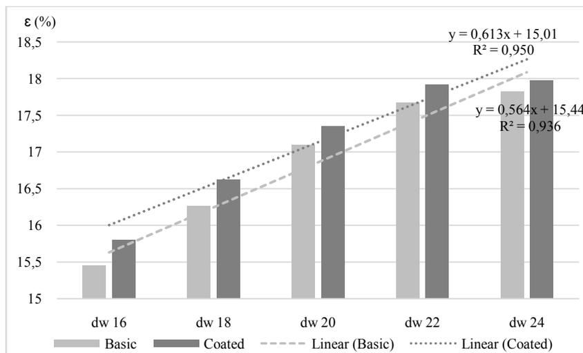
Fig.3. Elongation at break ( $\epsilon$  (%)) of tested fabrics - basic and coated fabrics, where: dw – warp density (threads/cm).
