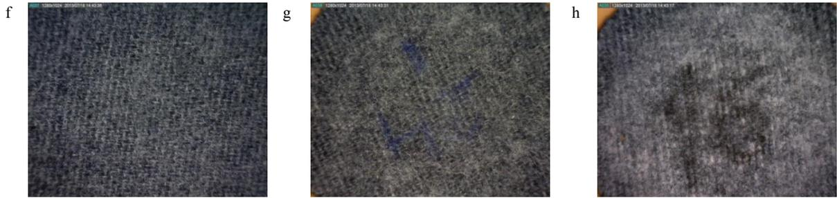
Fig. 10.(a) basic fabric before abrasion;(b) basic fabric after 100.000 abrasion cycles;(c) coated fabric before abrasion – face side;(d) coated fabric after 100.000 abrasion cycles – face side;(e) coated fabric after 400.000 abrasion cycles – face side;(f) coated fabric before abrasion – back side;(g) coated fabric after 100.000 abrasion cycles – back side;(h) coated fabric after 400.000 abrasion cycles – back side;(Dino-Lite Pro – AM-413T5).
