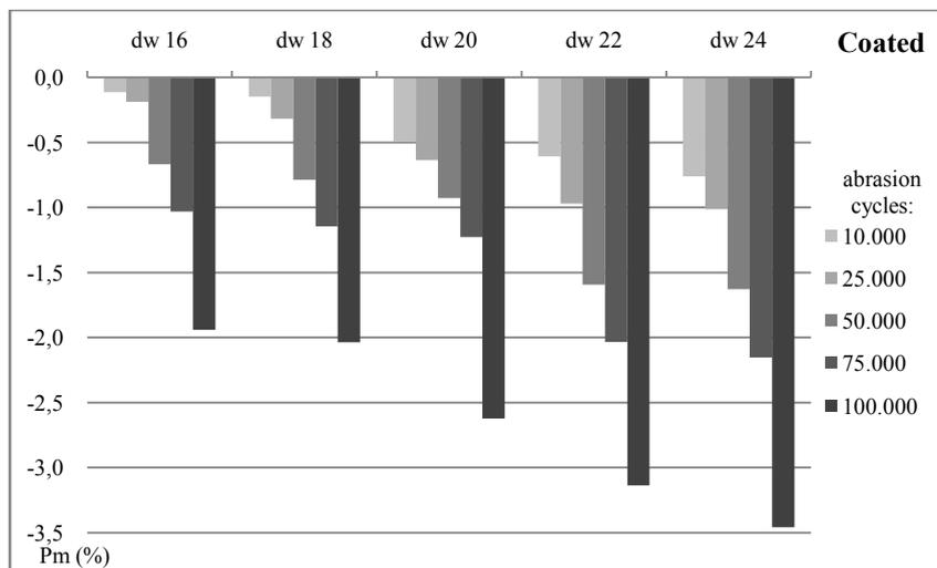
Fig.8. Abrasion resistance (Pm (%)) of tested coated fabrics, where: dw – warp density (threads/cm).
