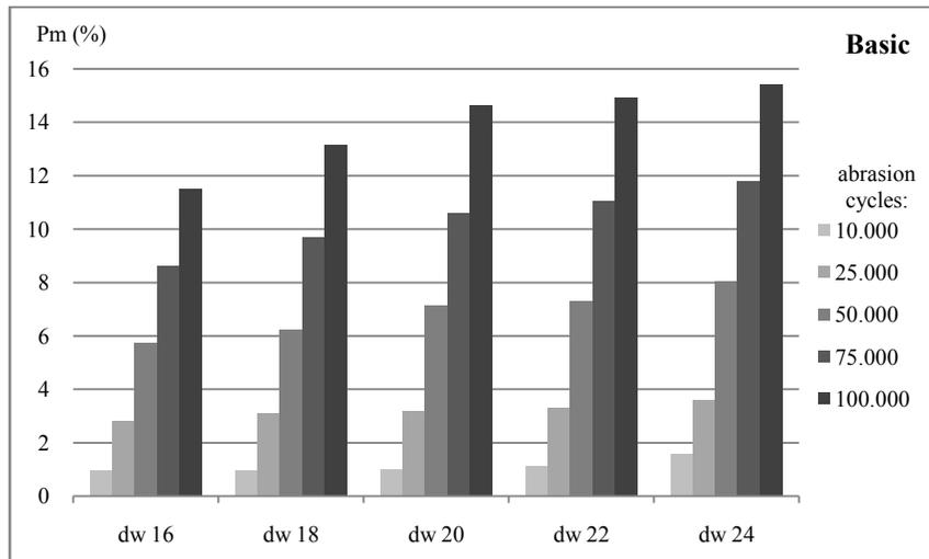
Fig.7. Abrasion resistance (Pm (%)) of tested basic fabrics, where: dw – warp density (threads/cm).
