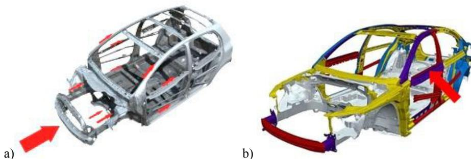
Fig. 2. The energy absorption at frontal (a) and lateral (b) impact.
