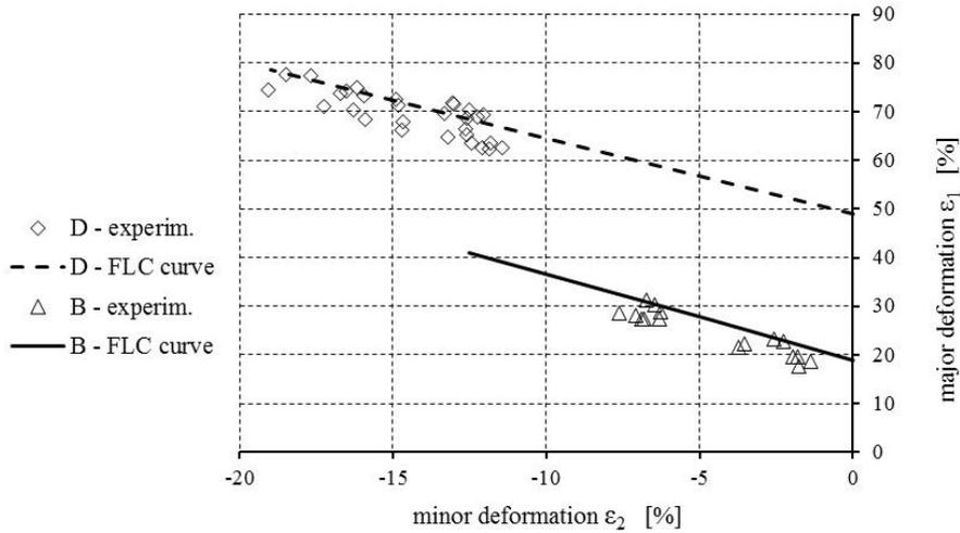
Fig. 7. Experimentally measured left part of forming limit curve.
