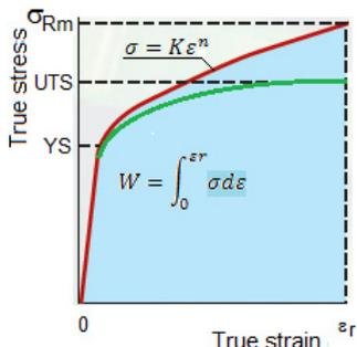
Fig. 3. True stress-true strain dependence.
