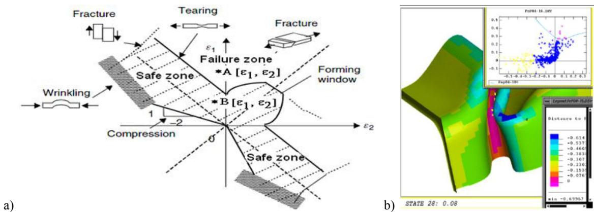
Fig. 4. Forming limit diagram [9] – (a) and result of FEM simulation of beam compression – (b).
