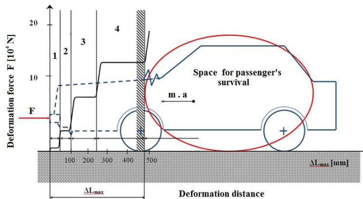
Fig. 1. Simple dynamic model of car at frontal impact to fixed wall
