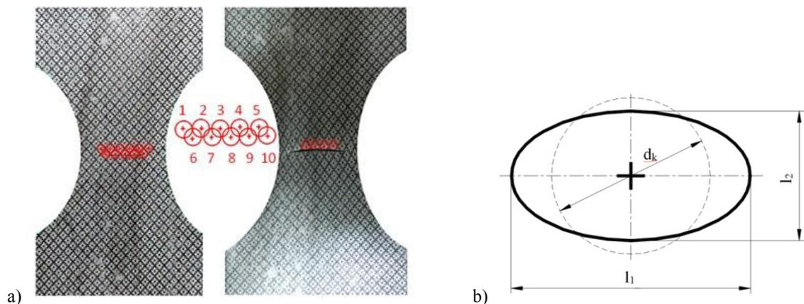
Fig. 5. Specimen with deformation grid before (left) and after (right) deformation – (a) and evaluation of deformed grid elements – (b).
