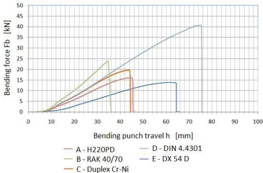
Fig. 9. The force-distance records at bending test.
