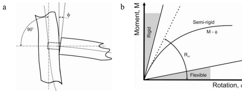
Fig. 1. (a) semi-rigid joint; (b) moment-rotation curves.
