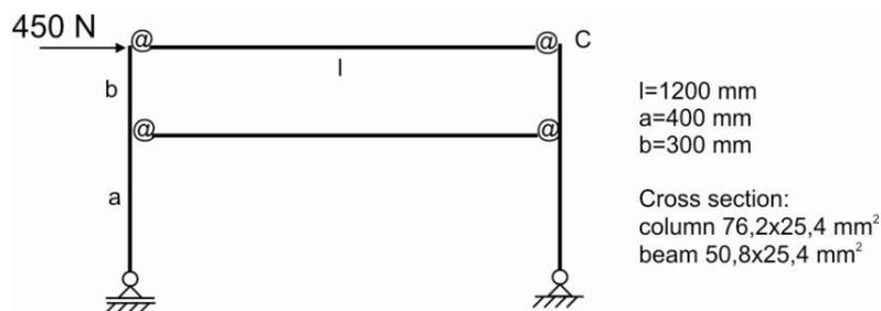
Fig. 7. Frame: physical model and loading diagram.
