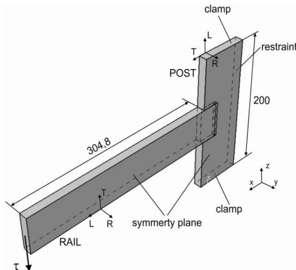
Fig. 3. Mortise and tenon joint loading diagram.
