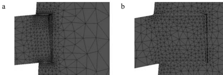
Fig. 4. Joint deformations: a) tenon length 12,7 mm, b) tenon length 50,8 mm, (symmetry plane; scale 20:1).
