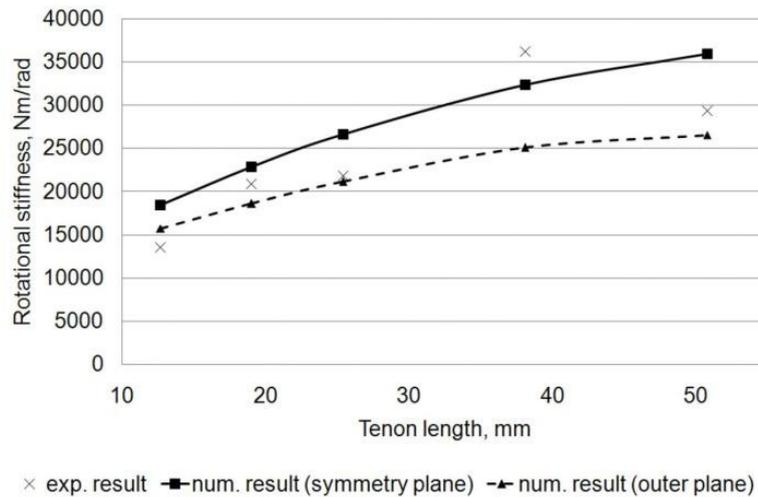
Fig. 6. Rotational stiffness R - five tenon lengths.
