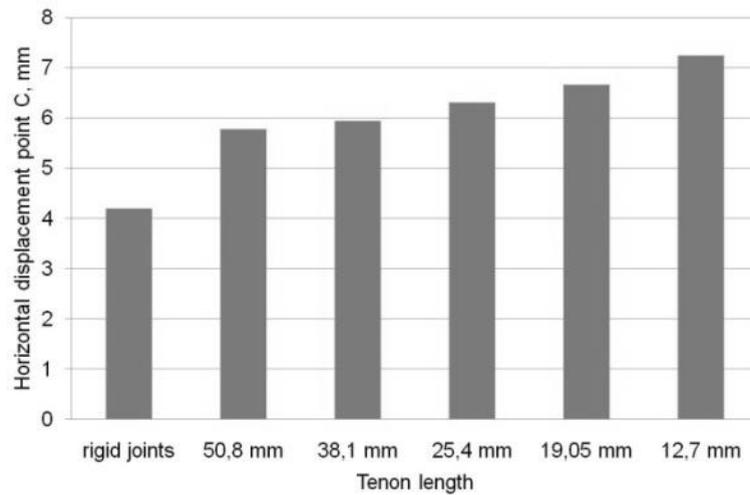
Fig. 8. Horizontal displacement point C for semi-rigid joints (five tenon lengths) and for rigid joints.
