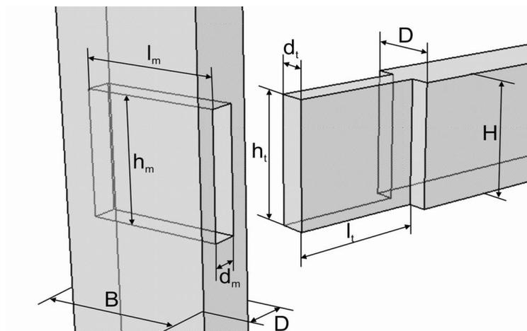
Fig. 2. Mortise and tenon joint geometries.
