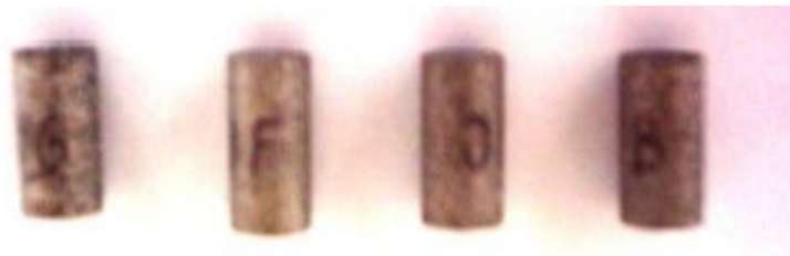
Fig. 2. Composite samples titan-5% hydroxyapatite.[3]
