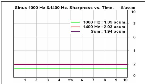
Fig. 11. The superposition of two tones with 1000 Hz and 1400 Hz: sharpness vs. time
