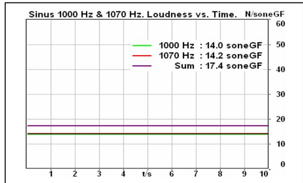
Fig. 6. The superposition of two tones with 1000 Hz and 1070 Hz: loudness vs. time
