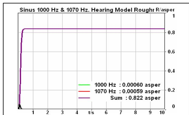
Fig. 8. The superposition of two tones with 1000 Hz and 1070 Hz: roughness vs. time
