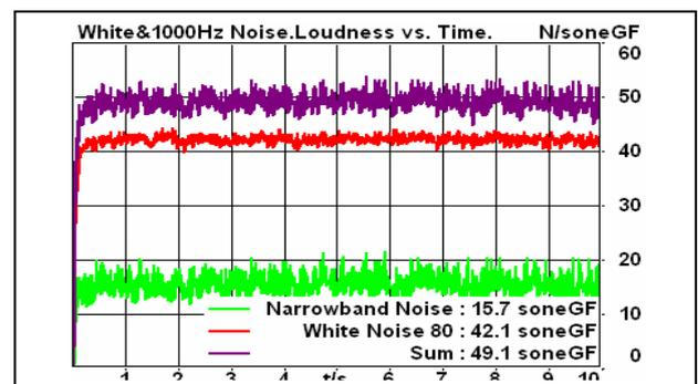
Fig. 2. The superposition of white noise and 1000 Hz narrow band noise: loudness vs. time
