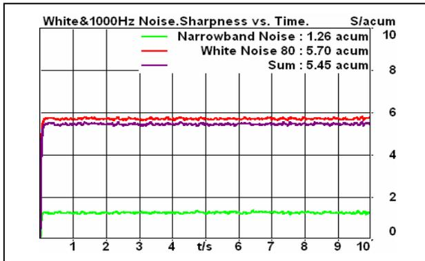
Fig. 3. The superposition of white noise and 1000 Hz narrow band noise: sharpness vs. time
