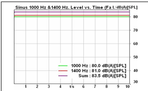
Fig. 9. The superposition of two tones with 1000 Hz and 1400 Hz: A-weighted level vs. time
