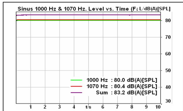
Fig. 5. The superposition of two tones with 1000 Hz and 1070 Hz: A weighted level vs. time
