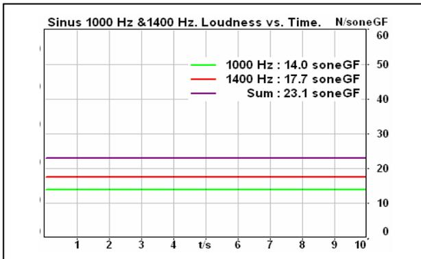
Fig. 10. The superposition of two tones with 1000 Hz and 1400 Hz: loudness vs. time
