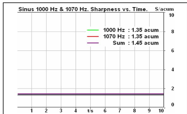
Fig. 7. The superposition of two tones with 1000 Hz and 1070 Hz: sharpness vs. time
