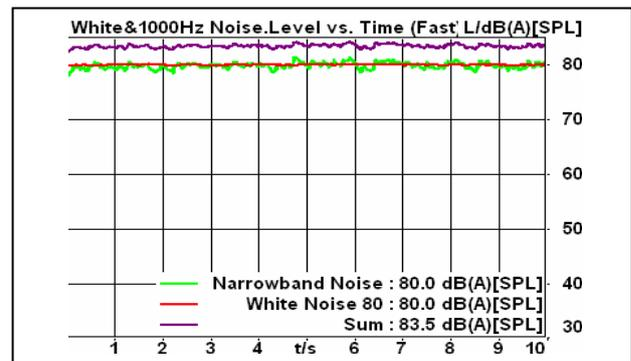
Fig. 1. The superposition of white noise and 1000 Hz narrow band noise: the A-weighted level vs. time
