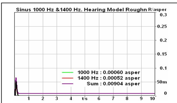
Fig. 12. The superposition of two tones with 1000 Hz and 1400 Hz: roughness vs. time
