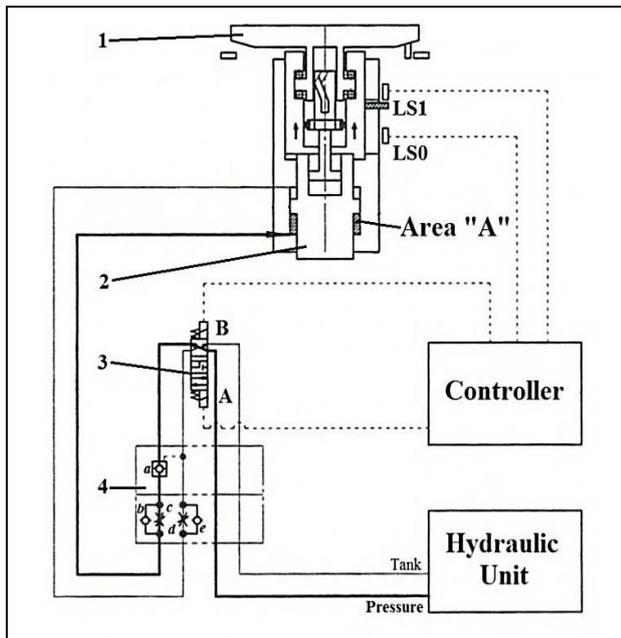
Fig. 3. Automatic Pallet Changer Arm Up Mechanism
