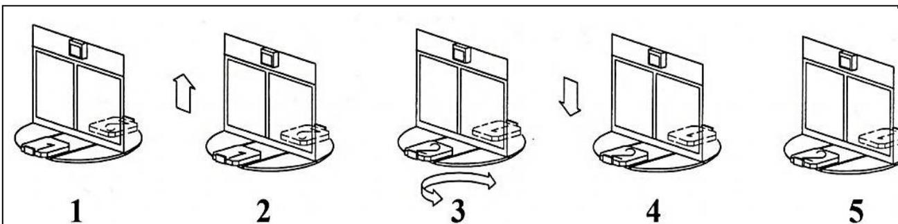
Fig. 2. Automatic Pallet Changer Operation Sequence
