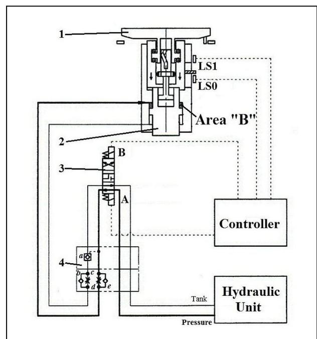
Fig. 4. Automatic Pallet Changer Arm Down Mechanism
