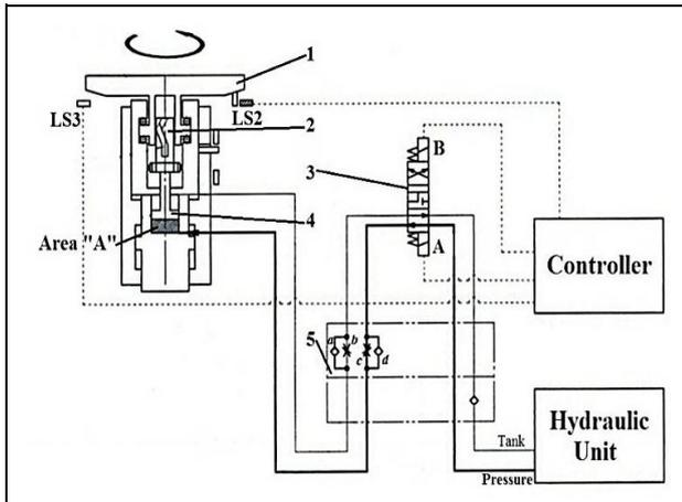
Fig. 5. Automatic Pallet Changer Arm Clockwise Rotation Mechanism
