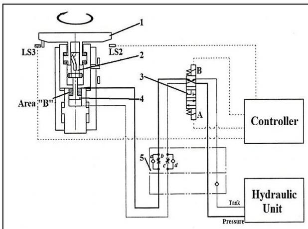
Fig. 6. Automatic Pallet Changer Arm Counterclockwise Rotation Mechanism
