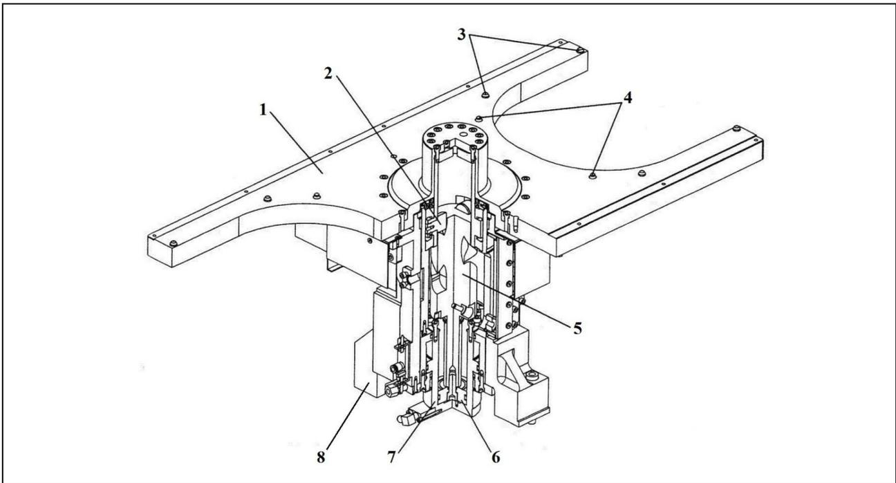
Fig. 1. Automatic Pallet Changer Mechanism
