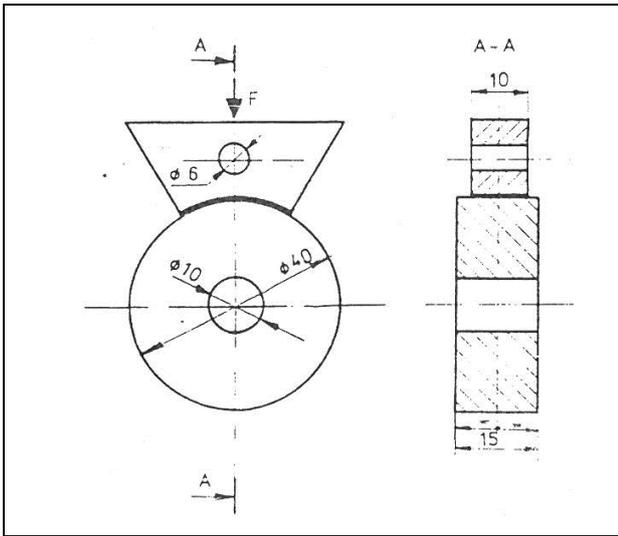
Fig. 2. Supporting pin - shoe assembly for wear test
