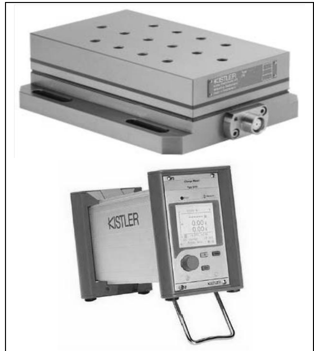
Fig. 3. The Kistler dynamometer system used for machining forces measurements
