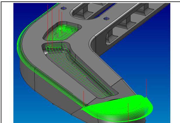
Fig. 5. Milling finishing exterior contour - tool routes
