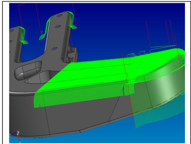
Fig. 6. Milling finishing exterior contour - tool routes
