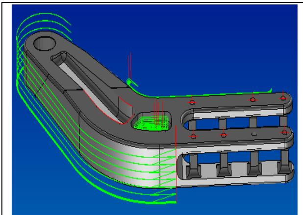
Fig. 4. Milling finishing pocket walls – tool routes
