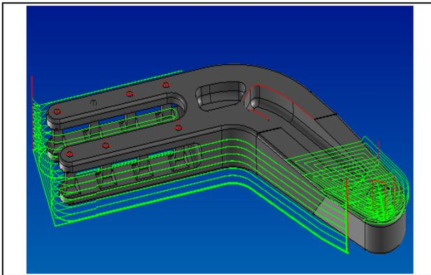
Fig. 3. Manufacturing the brackets – tool routes
