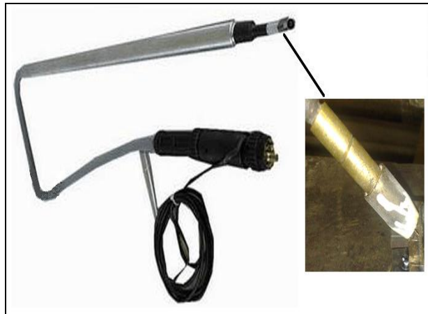
Fig. 3. Build-up welding torch [3, 6]
