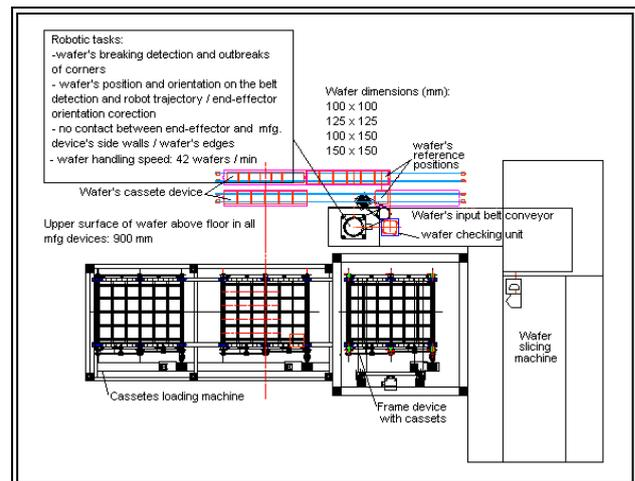
Fig. 1. Generic layout of wafer's flexible manufacturing line (partially view) including: wafer slicing equipment and transporting system - belt conveyor, robotized FMC for wafer diagnosis & loading into "cassettes" processing device, conveyors and special purpose machine for "cassettes" loading into "frame" processing devices
