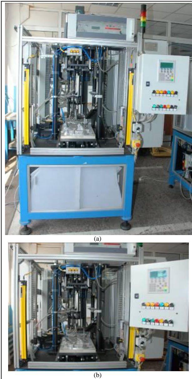
Fig. 3. (a, b) Adaptronics equipment for intelligent measurement for the tightness checking of distribution crankcase
