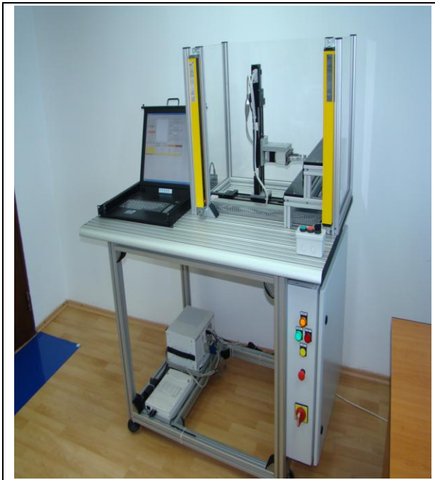
Fig. 5. Flexible adaptronics system for micro-measurement and micro-positioning for industrial micro-platform
