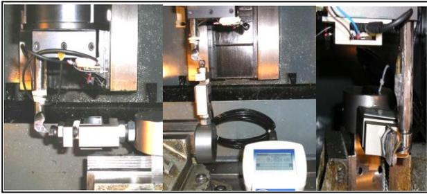
Fig. 5. Gauge sensitivity measurement test on three orthogonal directions
