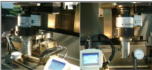
Fig. 6. Whole assembly stiffness characterization
