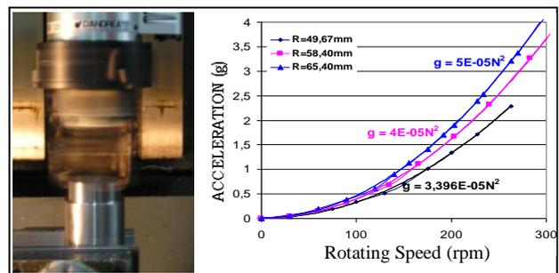
Fig. 9. Accelerometer response for the centrifugal force
