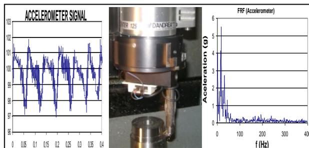
Fig. 10. Accelerometer signal in a non stable condition. Forced vibration case
