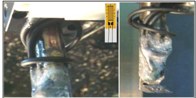
Fig. 7. Detail of the Gauge and Accelerometer embedded in the boring bar
