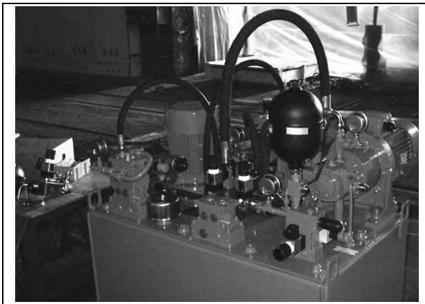
Fig. 8. Hydraulic unit for driving the semi-finished product clamping-unclamping
