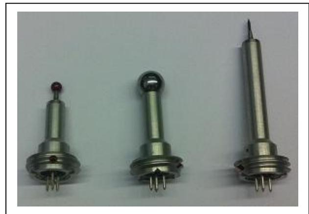
Fig. 2. Standard AACMMs probes (ROMER Sigma & Omega brands)
