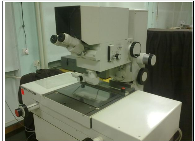
Fig. 4. The measuring of kerf width using ZKM universal two-coordinate microscope
