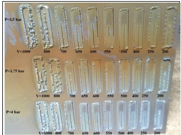
Fig. 5. The cut samples after plasma cutting low alloy steel with varying the cutting speed and the plasma gas pressure
