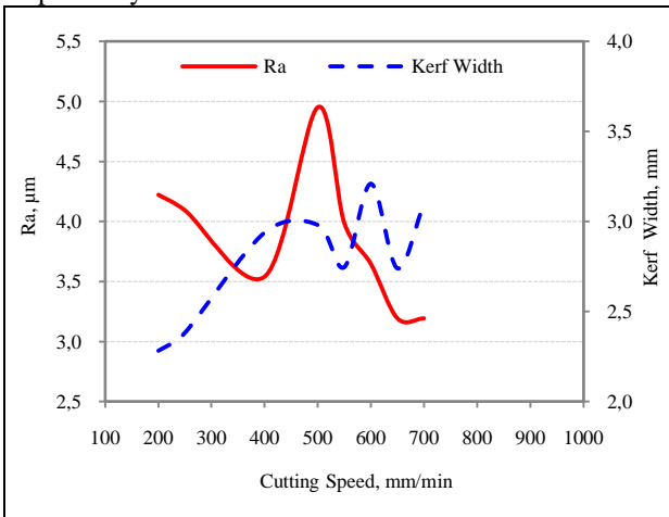
Fig. 6. The effect of cutting speed on surface roughness and the kerf width at a constant plasma gas pressure of 3 bar
