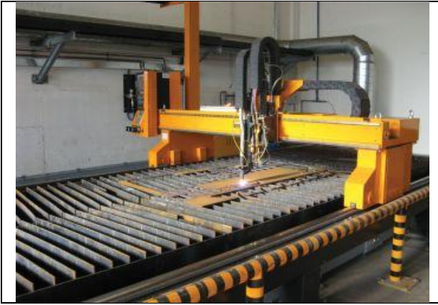
Fig. 1. CNC portal cutting machine VARCUT L2
