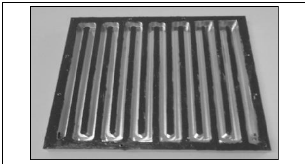
Fig. 3 Meandering inner surface of the heating plate
