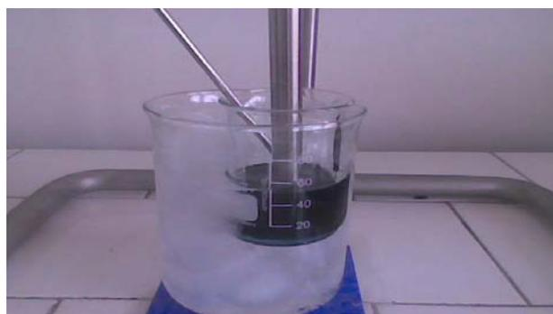
Fig. 1. The dispersion by ultrasonication process in polyester matrix
