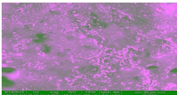
Fig. 5. SEM analysis of polyester/ MWCNT nanocomposite material (0,15% MWCNT)
