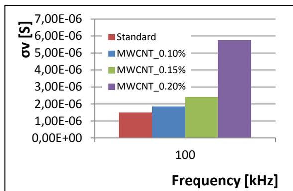
Fig. 2. Variation of volume electrical conductivity depending on MWCNTs concentration
