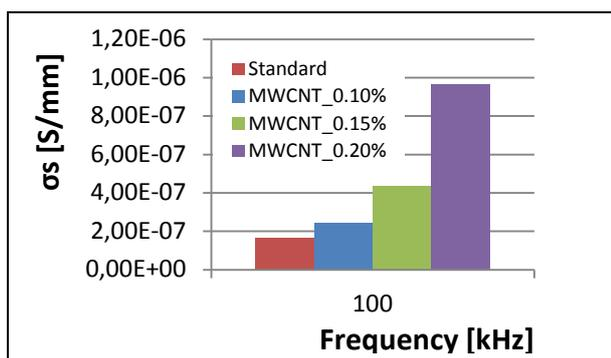
Fig. 3. Variation of surface electrical conductivity depending on MWCNTs concentration
