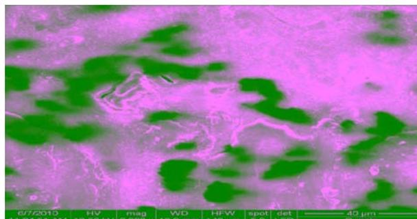
Fig. 6. SEM analysis of polyester/MWCNT nanocomposite material (0,20% MWCNT)
