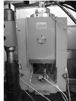
Fig. 7. Real model of hydraulic unit with strain gauges and eccentrically placed dynamometer
