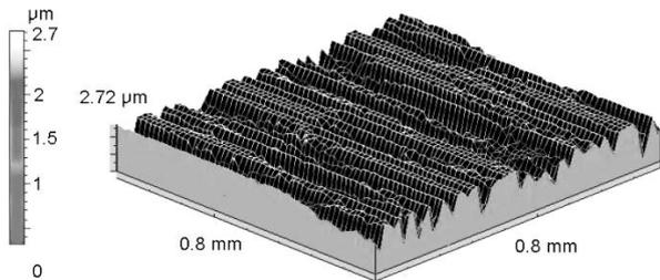
Fig. 3. 3D surface roughness of underlying surface
