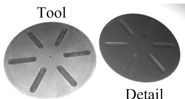
Fig. 2. Rubber pad forming tool and detail
