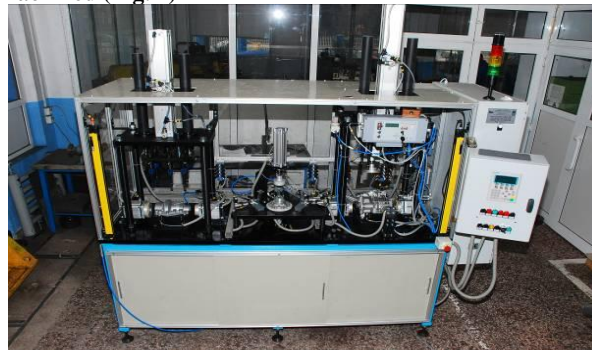
Fig. 2. Intelligent machine for dimensional control and marking
