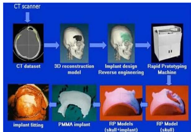
Fig. 1. Generalized procedure for creating medical models
