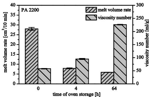
Fig. 2. MVR and viscosity number measurements of PA12 powder
