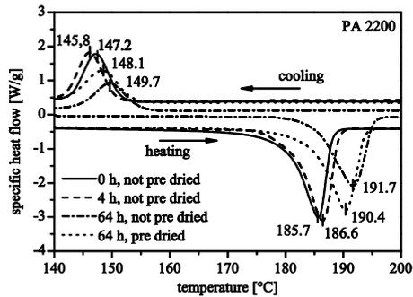
Fig. 1. DSC measurements of PA12 powder
