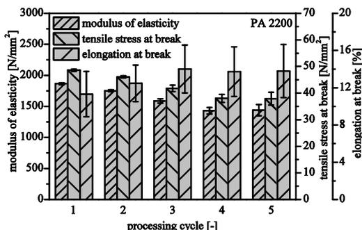
Fig. 3. Mechanical properties of laser sintered parts (ca. 5h / cycle)
