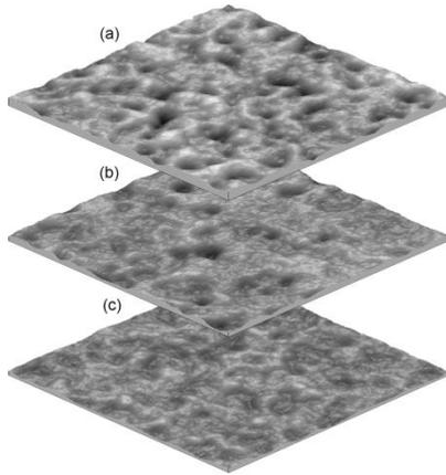
Fig. 1. Continuous 3D Axonometric Representations of the Surface Profile of Components Manufactured at Laser Powers of (a) 3 W, (b) 4.5 W and (c) 8 W
