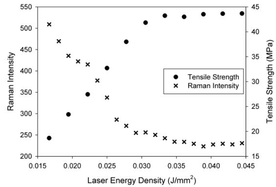
Fig. 3. Graph Showing Raman Intensity and Tensile Strength Versus Laser Energy Density
