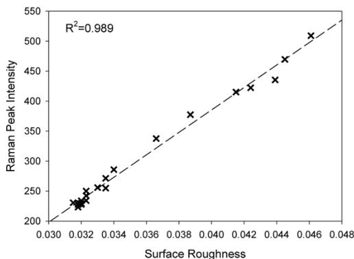
Fig. 2. Graph to Show Linear Relationship Between Raman Peak Intensity and Surface Roughness
