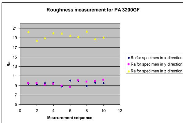
Fig. 4. Roughness distribution for all three directions
