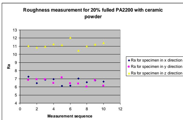
Fig. 5. Roughness distribution for all three directions
