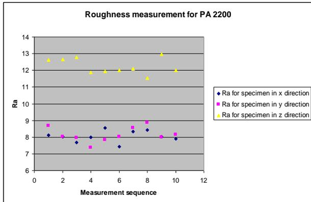
Fig. 3. Roughness distribution for all three directions
