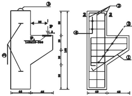
Fig. 1. Experimental element – form, dimensions, fixture
