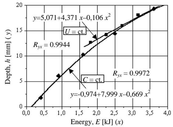
Fig. 4. Dependence of forming depth on the energy, for  $U=ct.$  and  $C=ct.$
