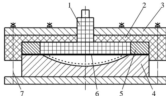
Fig. 2. Scheme of experimental tools: 1- flat spiral coil; 2- wooden casing; 3- fixing plates; 4- forming die; 5- ring; 6- workpiece; 7- tightening screws
