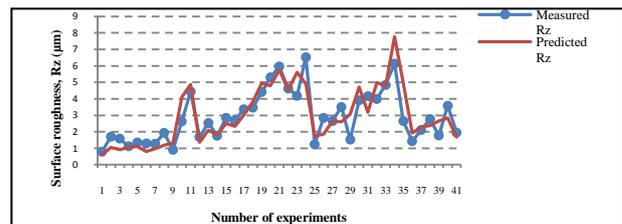
Fig. 3. Example of the measured surface roughness and the predicted surface roughness,  $R_z$
