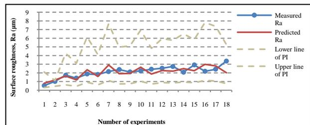
Fig. 4. Example of the measured surface roughness, the predicted surface roughness, and the 95% prediction interval of the predicted surface roughness,  $R_a$
