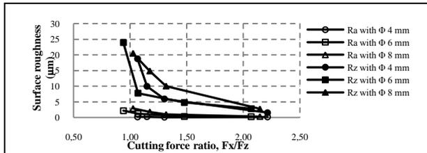
Fig. 2. Examples of experimentally obtained relations of surface roughness, and cutting force ratio at  $V$  10,000 rev/min,  $f$  0.03 mm/rev,  $D$  0.3 mm
