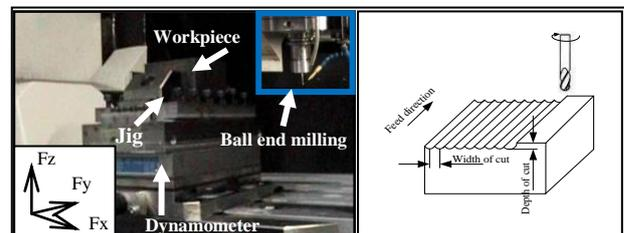
Fig. 1. Illustration of the experimental setup and the feed direction of the ball end mill
