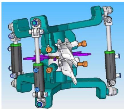
Fig. 1. Mechatronic device that simulates the relative motion between two lumbar vertebrae and measures the inter vertebral pressure.
