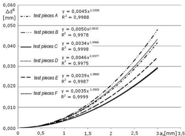
Fig. 2. Relationship between diameter deviation  $\Delta d^s$  of various test pieces from cutting depth  $a_p$ , determined in relation to reference cylindrical surface diameters of each piece.
