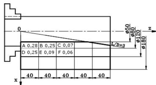
Fig. 1. Normalised weight coefficients in representative elementary machining zones (A-F)
