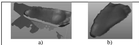
Fig.5. The procedure of obtaining the foot CAD model by scanning, using the laser beam 3D handy scanner: a) the filtering of model's intermediate image; b) final model
