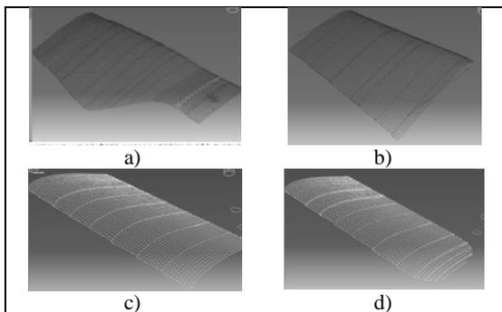
Fig. 3. The CAD models for each equidistant scanned zone portioned from the blade's 1<sup>st</sup> lateral surface: a) zone 0-1; b) 1-2; c) 2-3; d) 3-4
