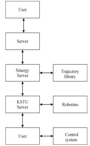
Fig. 1. Structure of the remote access
