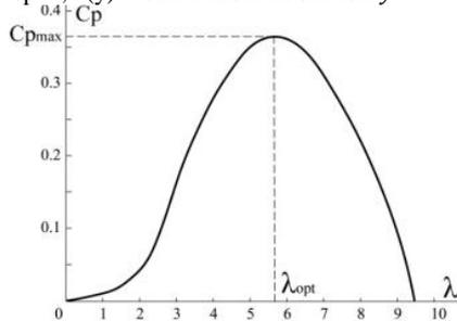
Fig. 1. Power coefficient variation  $C_p$  depending on the end speeds ratio  $\lambda$
