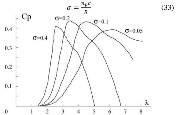
Fig.2. Influence of  $\sigma$  solidity ratio on the  $C_p(\lambda)$  curve
