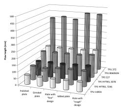
Fig. 5. Dependence of the flow length on the injected material (injection rate 60 mm.s<sup>-1</sup>, injection pressure 80 MPa)
