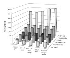
Fig. 4. Dependence of the flow length on the injected material (injection rate 60 mm.s<sup>-1</sup>, injection pressure 60 MPa)
