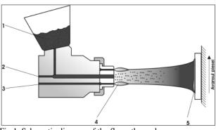
Fig.1. Schematic diagram of the flame thermal spray process and powder. 1-powder, 2-input powder, 3-gas mixture, 4-flame, 5-layer deposited by thermal spray. (Iovănaş, 2006)
