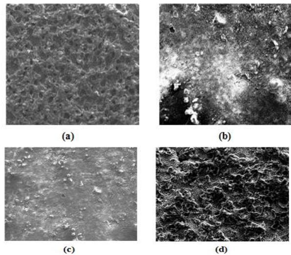
Fig. 2. SEM micrograph of SiCp/6061 aluminum MMC after WEDC at (a) servo voltage 70 V; (b) servo voltage 90 V; (c) pulse-on time of 1 μs; (d) pulse-on time of 4 μs;
