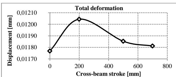
Fig. 4. Total deformation dependence of cross-beam stroke
