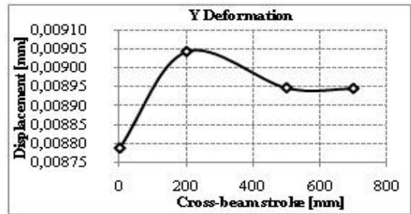
Fig. 6. Y deformation dependence of cross-beam stroke
