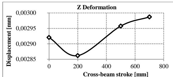
Fig. 7. Z deformation dependence of cross-beam stroke
