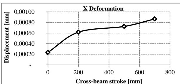
Fig. 5. X deformation dependence of cross-beam stroke
