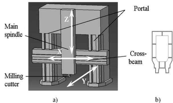
Fig.1. a) 3D model of the portal machine b) the diaphragm section of the columns
