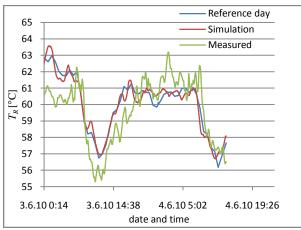
Fig. 1. Experiment results (comparison of return temperatures)
