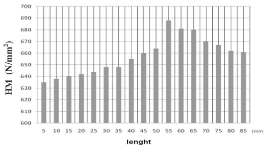
Fig. 4. Evolution of Martens hardness depending on symmetry axis of the crystal
