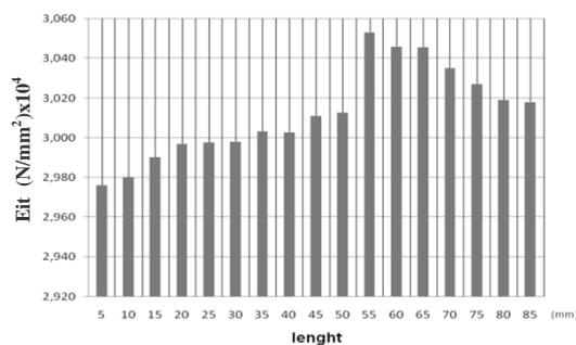
Fig. 5. Evolution of elasticity modulus depending on symmetry axis of the crystal
