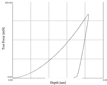
Fig. 2. Cyclogram of Martens loading-unloading
