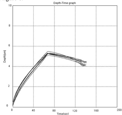
Fig. 6. Evolution of the creep measured in different points on the cadmium telluride crystal constant load of 500 mN and times of stress 15 seconds
