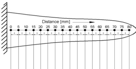
Fig. 3. Measuring of mechanical characteristics of resistance, positions and distances on cadmium telluride crystal
