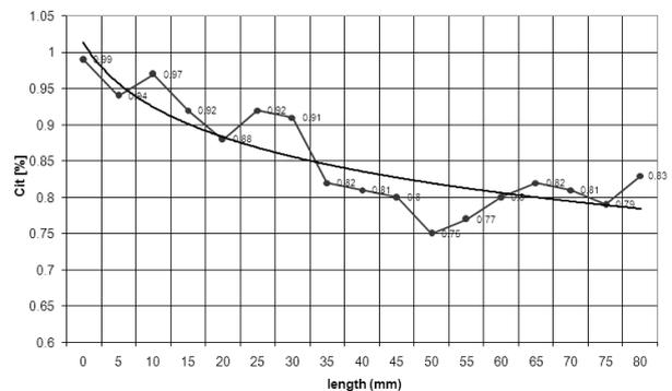
Fig. 7. Variation of maximum indentation depth under load (creep trend) determined at different measuring points on the cadmium telluride crystal to a time test of 15 seconds
