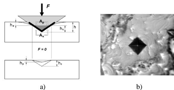
Fig. 1. a) the main geometrical characteristics in Martens hardness testing and instrumental hardness test, b) after removal of indenter from the tested material
